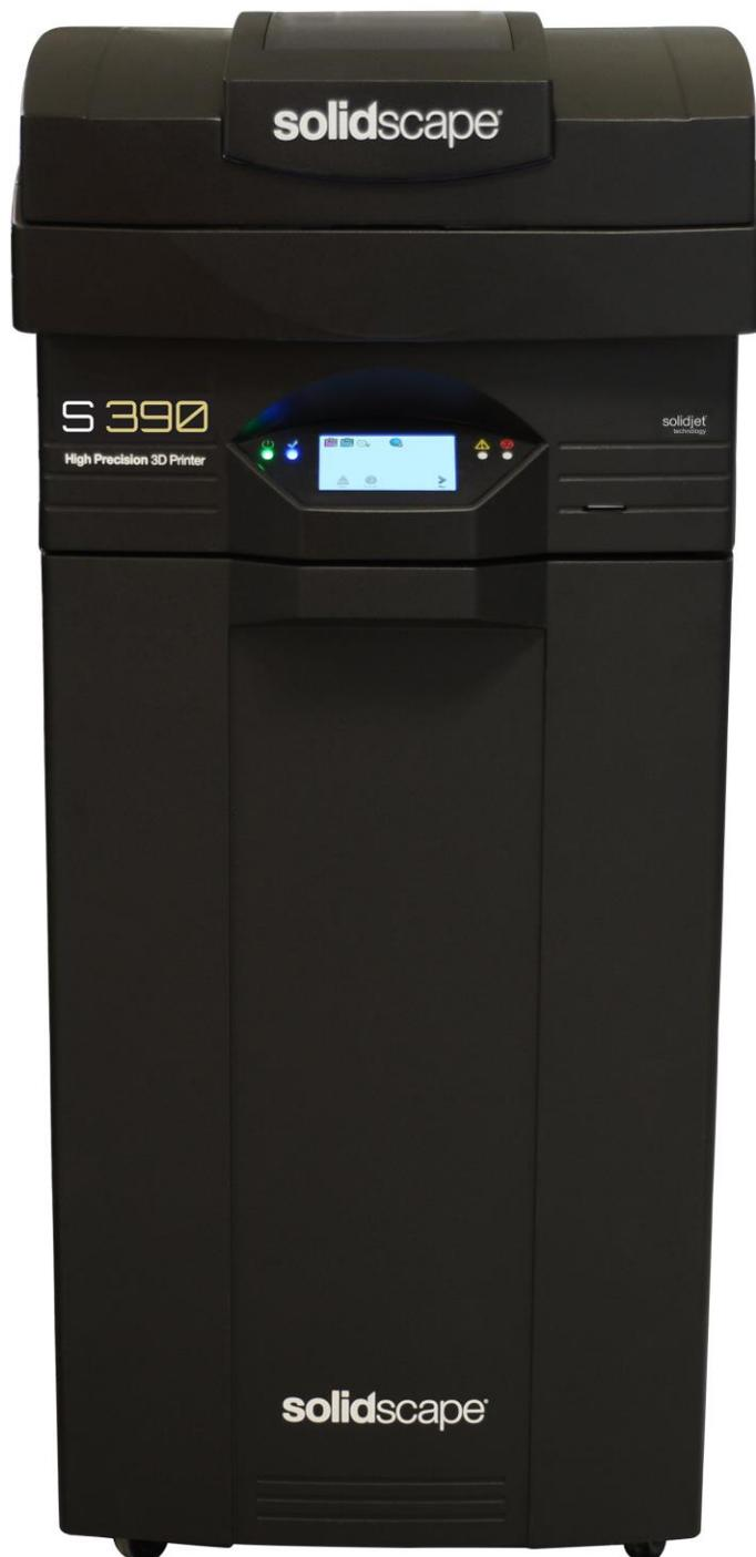
The S390 high precision 3D printer features Solidjet technology that optimizes how Solidscape prints castable patterns, powering the same Solidscape precision even faster. The total system includes a Solidscape base and industrial dust collection system.
