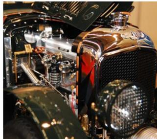
Casting for critical components was undertaken by Horbach GmbH based from models created on SolidScape machines. Precision was of paramount importance for the model’s many moving parts such as workable brakes, clutch, choke and adjustable ignition.
